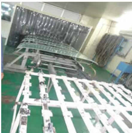
De-airing for bus and truck glass
