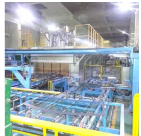
Bending furnace for car glass
