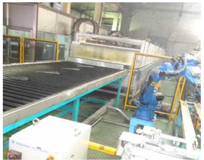
Tempering for sildelites (side glass)
